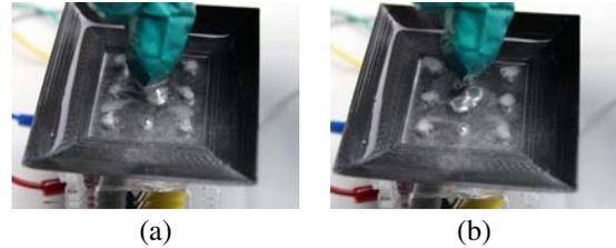
Figure 3. A JDLED pixel is deforming between spherical and flat shapes in response to an appropriate DC voltage to provide tactile sensation.
